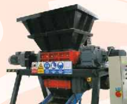
DR240/900_37kW Machine intended for heavy-duty operating conditions. Shreds plastics, wood, tires, etc.
